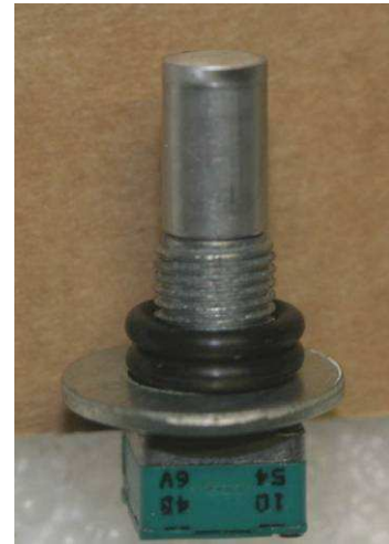
Photo shows the metal spacer washer with two spacer rings on a potentiometer.
