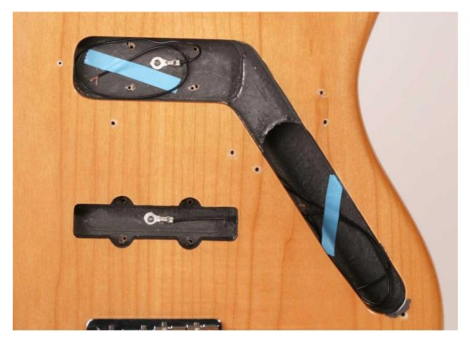
The goal was to develop a cancelling coil which was much smaller than a normal pickup to fit into this routed wire pathway which could cancel the noise from most types of single coil pickups across a wide range of frequencies and include it with the preamp for a price players could afford – gulp.
