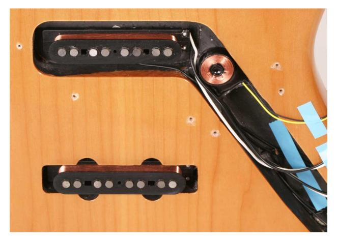
A lot of development effort went into making this work, for example, we had to design unique custom measurement equipment and acquire an amazing number of measurements on different pickups. The noise sensors use different sensing coils created on a computer controlled winding machine to match, by pickup type, the amplitude and phase response across the frequency range.
