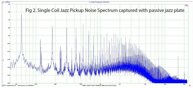
This looks ugly! The traditional hum bucker was designed 60 years ago and did a good job at cancelling 50/60 cycle power line noise and the first few overtones which were the main problems at that time when the number of significant overtones were limited due to "soft" tube diodes.
