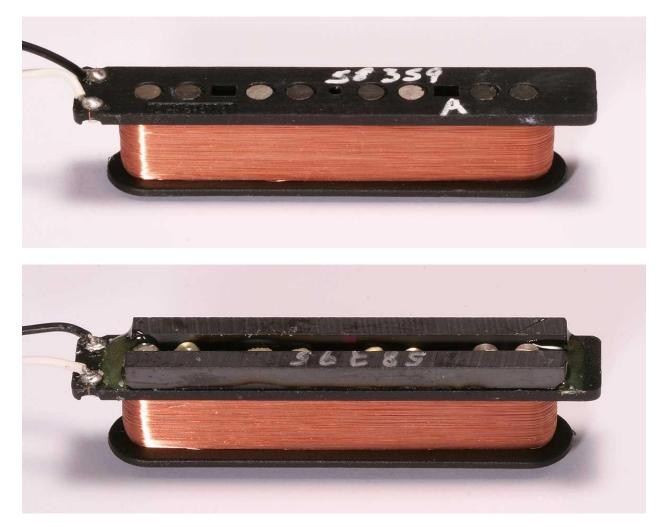
Most ceramic pickups and the pickups containing the rare earth magnets (samarium cobalt or neodymium) use steel pole pieces, sheets or bars to control the shape of the magnetic field. In the common configurations this steel also causes the pickups to collect more noise than AlNiCo pickups.
