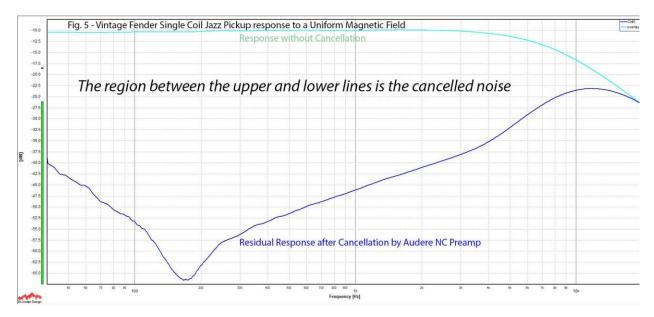
Remember that 10 dB is 10 times the power – so each 4 horizontal graph lines are 10x the power level. The top teal line is the amplitude of noise collected vs. frequency for this Jazz Pickup. The Blue line is the residual response after the cancellation by our preamp. Lower on the graph is better for the blue line but what is important is the difference in between the 2 lines.
