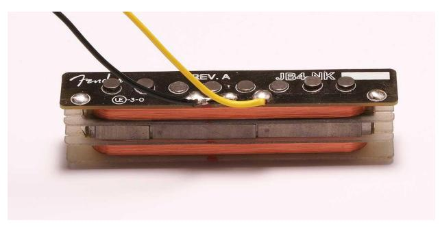
The 2 coils are wired out of phase with each other and might or might not have equal windings. Depending on the magnetic system design the bottom coil may add a significant volume to the strings response but often is assumed to be non-sensitive to the string's vibration.
