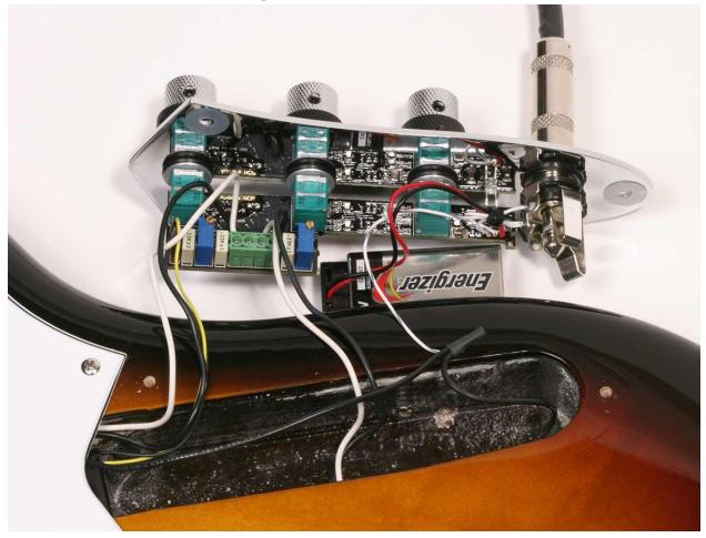
The preamp front end signal path is a stereo design. Each pickup input has a dedicated signal path. The noise sensor signal is processed as a 3rd input and does not compromise the sound of the pickups. The noise sensor's gain is adjusted independently for each pickup by 2 trim pots. These trim pots are each 20 turns going from the max positive gain through 0 to the max negative gain (i.e. inverting the phase). Adjusting these pots for noise cancellation is easy:
