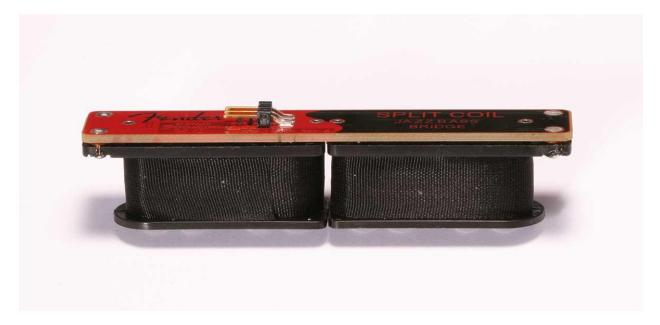
In the case of a 4 string bass the E & A strings share one coil and the D & G strings share a 2<sup>nd</sup> coil. The magnets and winding in the 2 coils are reversed.
